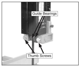
Figure 26. Front of upper blade guide.
